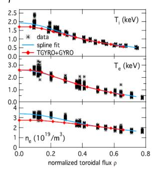
Simulation results (red) versus experimental data (blue) for ion temperature (top), electron temperature (middle) and electron density (bottom) and electron (right) for DIII-D L-mode discharge 128913. The TGYRO solutions in red represent a steady-state scenario in which measured input power and particle source balances the neoclassical and turbulent fluxes.
