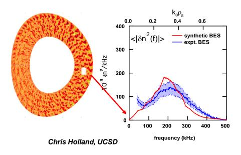
Visualization of turbulent density fluctuations from a firstprinciples gyrokinetic simulation of plasma turbulence and predicted fluctuation spectra
